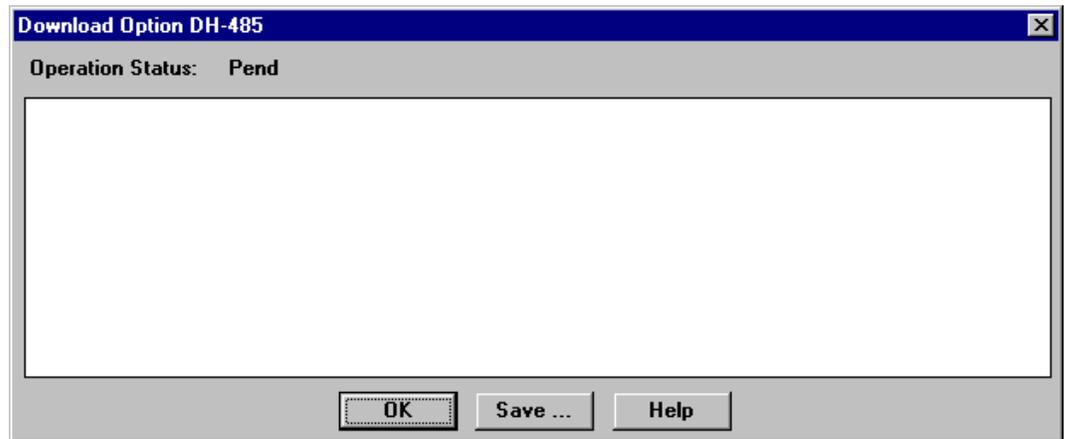
The Operation Status dialog box contains a list box of errors and/or status messages associated with a particular operation. Some of the errors or messages are about failed operations, while other errors or messages contain helpful information about successful operations. A status (Fail, Pend, or Pass) of the operation is also displayed.
