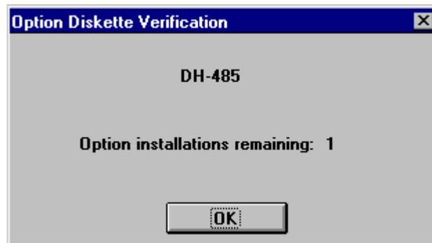
The **Option Diskette Verification** dialog box displays the option name and the number of remaining option installations. If you do not have any remaining installations, call the Cutler-Hammer Customer Support Center for assistance.
